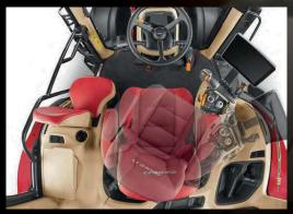
The AFS Pro 1200 is the primary display on the Magnum™, Steiger® and Optum® series tractors. The large 12-inch display features an easily customised touch-screen with Bluetooth® capabilities, superior HD visibility, day or night, and a familiar Android-based interface is just like using a smartphone or tablet.
